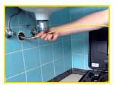
With this convenient camera complete system you can inspect easily all pipes from rooftop to basement. The flexible Mini Color Camera (23mm Dia.) can be pushed up to 30m with the glasfiber rod into the drain line and produces a detailed video picture of the internal condition of the pipe. The RKS110D is a perfect unit for all in-
