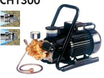
CH13OO for Pipes to 150mm Dia. with 230 V electric motor 2,2 kW, 13A,130 bar/11,41/min., high pressure drain hose 1/4" ID x 20m, Safety Foot Pedal, Penetrating Nozzle, Flushing Nozzle, Spray Wand w/10m HP hose. Code 56141
